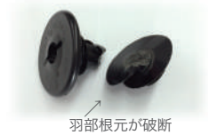
羽部根元が破断
